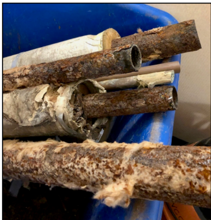
Old rusty riser pipes removed from Building 5. (Photo courtesy Al Fuentes)
